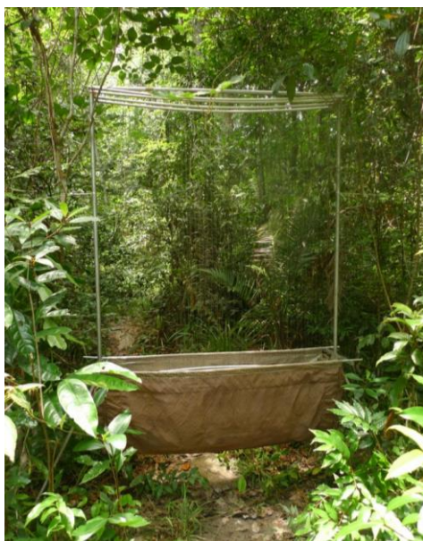
Fig. 2: Four-bank harp trap
